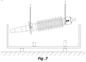
Lifting rope must be fixed under metal head and the beginning of hollow insulator, but never crushing silicone sheds.
