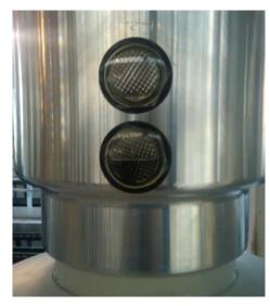
Fig. 2 - Prysmatic oil level indicators
